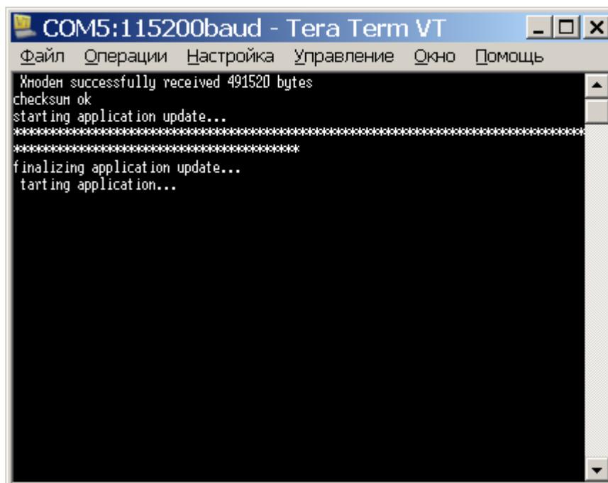
The image shows a screenshot of a Tera Term VT terminal window. The title bar reads "COM5:115200baud - Tera Term VT". The menu bar includes "Файл", "Операции", "Настройка", "Управление", "Окно", and "Помощь". The terminal output shows the following text:
